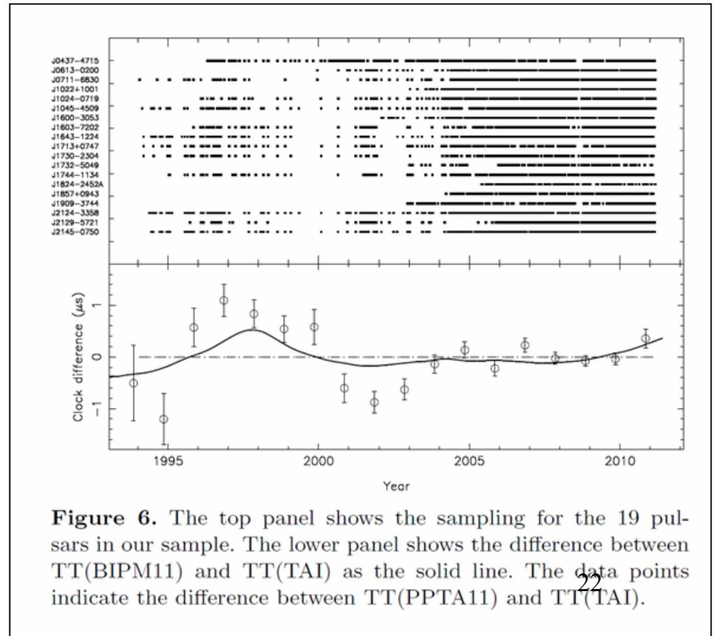
**Figure 6.** The top panel shows the sampling for the 19 pulsars in our sample. The lower panel shows the difference between TT(BIPM11) and TT(TAI) as the solid line. The data points indicate the difference between TT(PPTA11) and TT(TAI).
